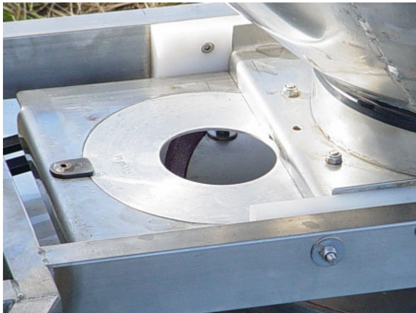
Fig. 11. Adjustable bait flow rate aperture.
