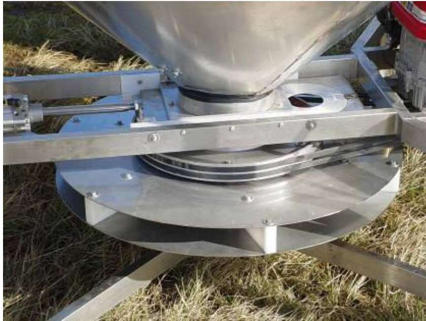
Fig. 12. Base of bucket shown with spreader mechanism (spinner) which is powered by lawn mower motor mounted on the side of the bucket. The slide holding the aperture ring shown in Fig. 10 is operated hydraulically by the pilot to allow bait to flow at the required time. This photograph shows the slide in the closed position and no bait would flow from the bucket to the spreader.
