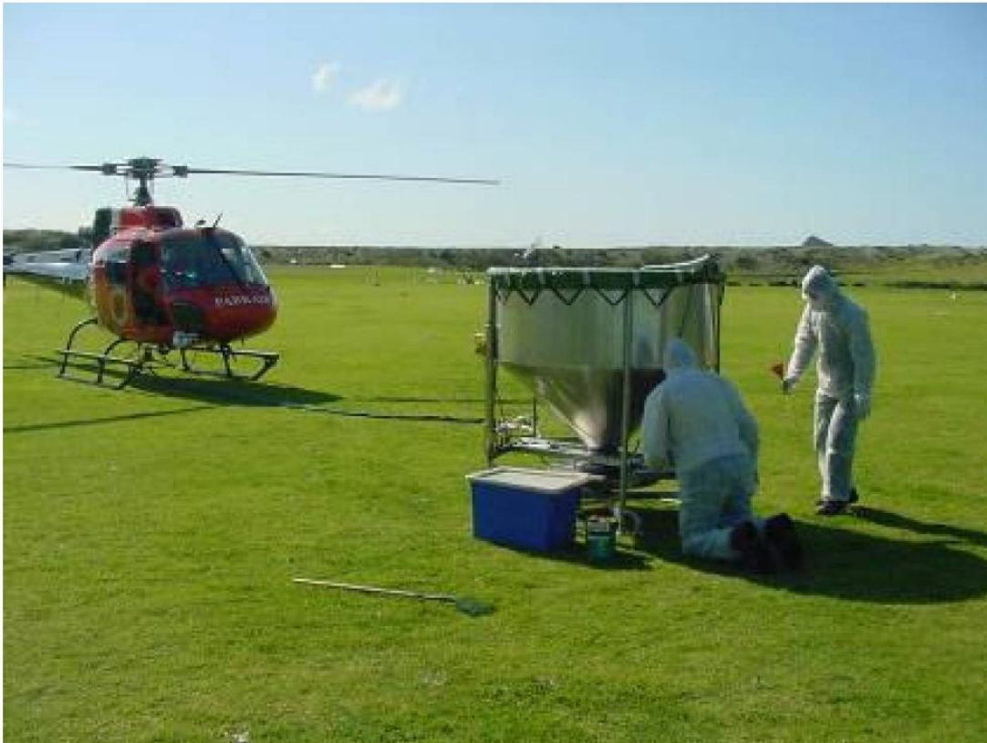
Figure 1: Custom built spreader bucket being prepared on LHI.
